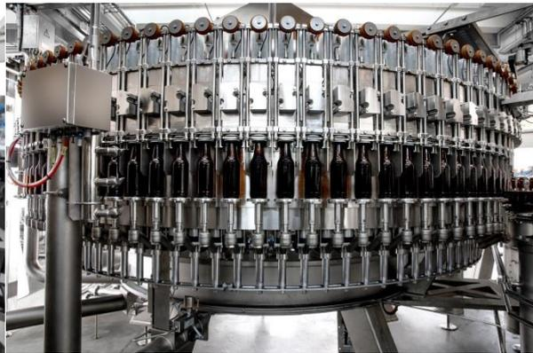
EvoFILL Glass has been engineered according to top hygienic standards. Its “no base” architecture results in easier operations during production and maintenance, while helping manufacturers deliver the highest quality products to their consumers.
