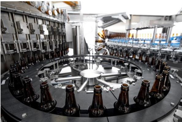
The re-designed handling parts, which are now lighter and smaller, ensure a changeover time shorter than 30 minutes with one operator.
